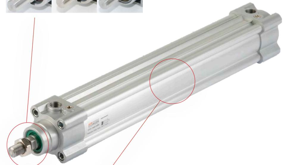
**HEART:** The piston, the heart of the cylinder and always subjected to intense work, must ensure a constant and lasting precision in any condition. It was therefore chosen to make it entirely of aluminium with a special anti-wear guide band to make it indestructible, precise and performing even after years of intensive use and with strong temperature variations.
